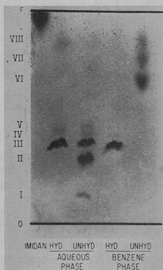
Figure 3. Chromatographic behavior of water- and benzene-soluble rat urinary metabolites of Imidan-C 14 for 12- to 24-hour interval, pre- and postacid hydrolysis
